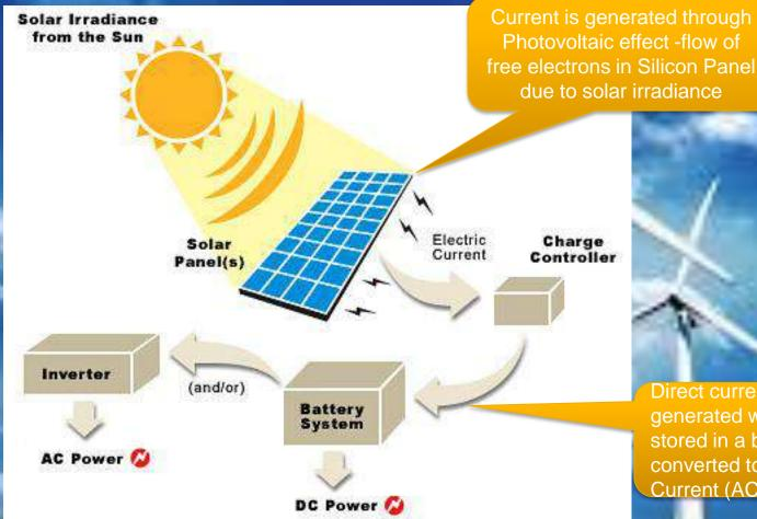
Direct current (DC) is generated which can be stored in a battery or converted to Alternating Current (AC)
